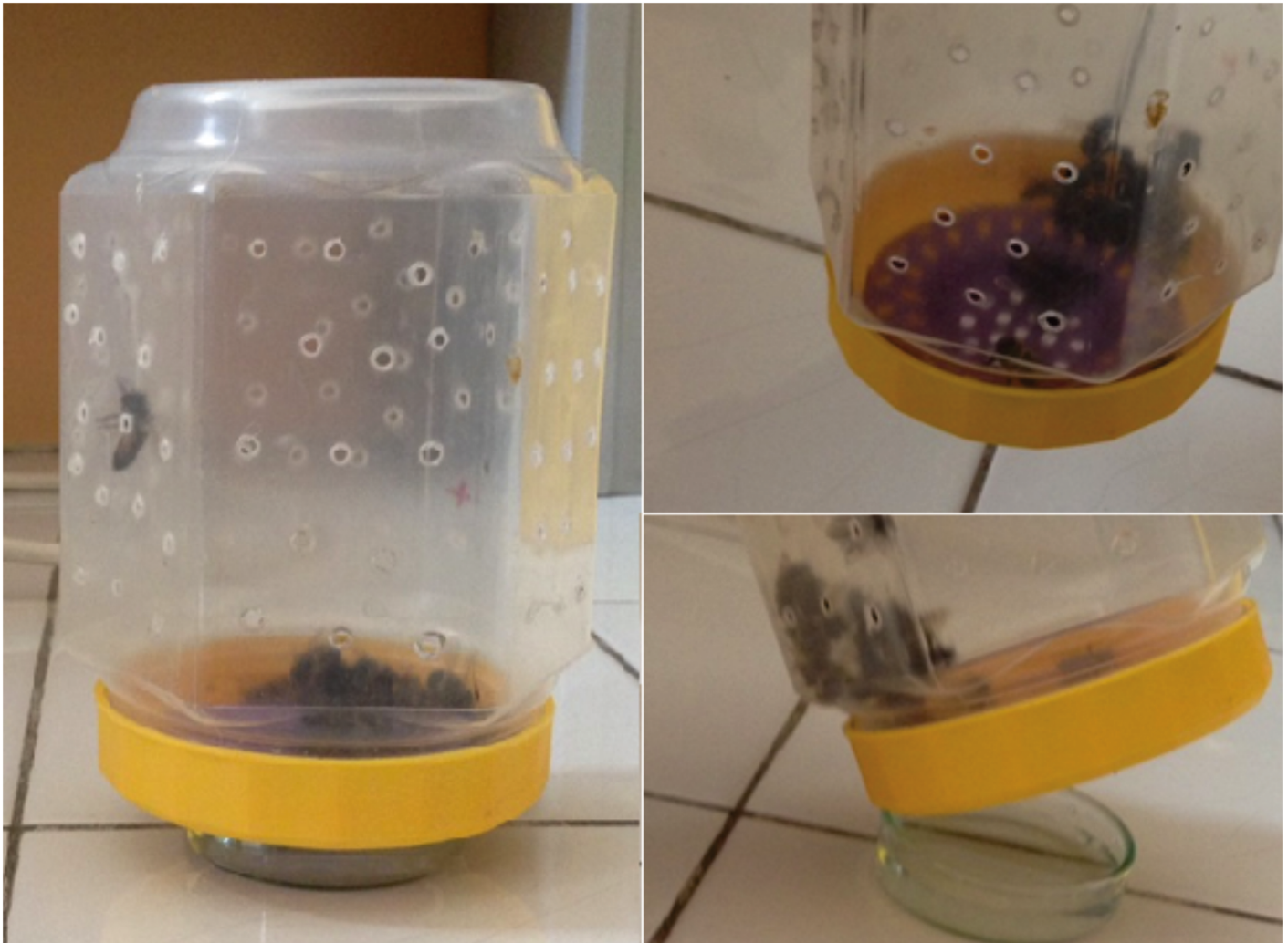
Fig 1. The modification of a laboratory cage: A plastic jar with small holes made for aeration and a plastic mesh sink strainer inserted into the lid allowing bees to take the food from a small petri dish placed below.
