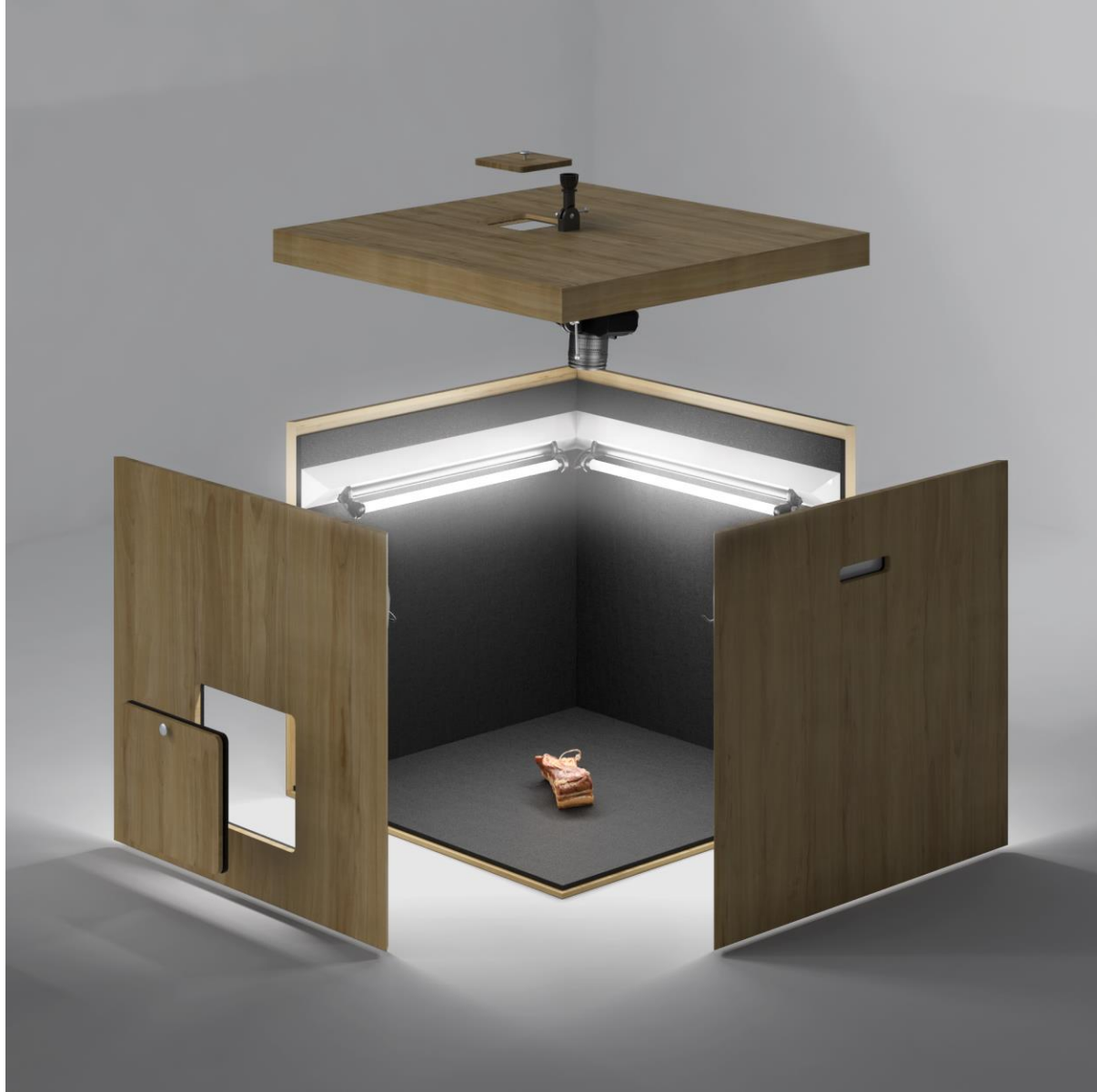
Fig. 1. Computer vision (image acquisition) system
