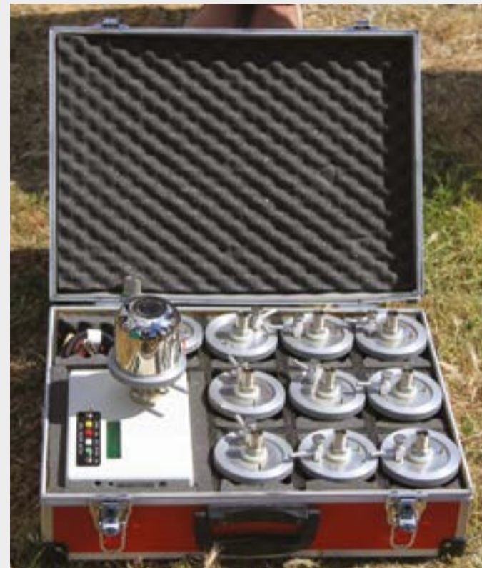
••• Instruments for collecting soil-gas samples, Ciudad Rodrigo 2016 exercise, Spain. Source: Tore Tollefsen.
