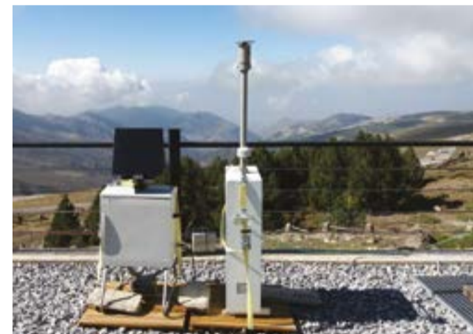
High-volume air sampler located at 2550m in Sierra Nevada, Spain, in the framework of the FRESA Project (CGL2015-70741-R). Source: FRESA Project.
