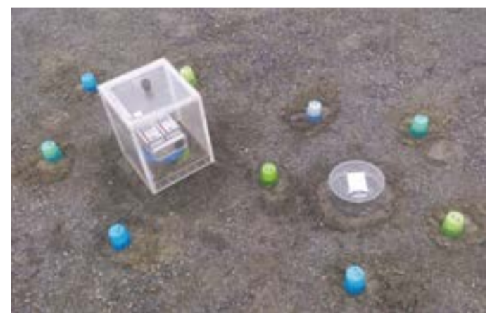
Radon exhalation rate measurements, Ciudad Rodrigo, Spain. Accumulation method using active monitors and charcoal cartridges (inside the plastic glass). Source: Luis S. Quindós.
