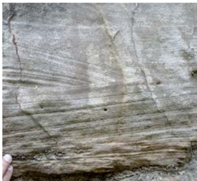
Cross-bedded sandstone used as a block from a retaining wall. Source: Roberto Braga.
