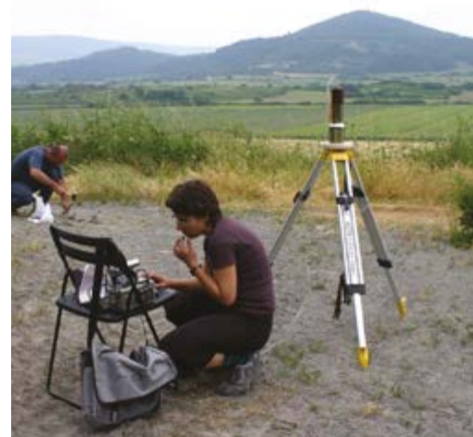
••• A NaI detector placed one metre above the ground. Source: Laura Tositti.
