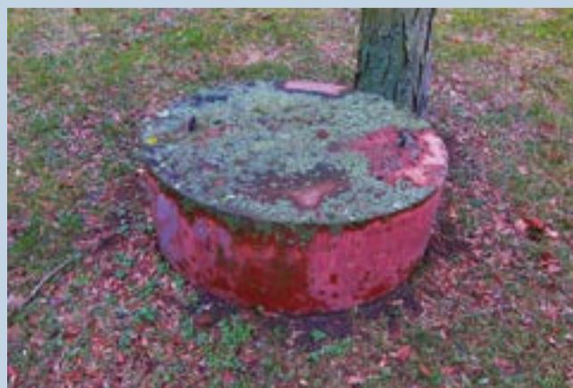
••• Calibration pads, concrete enriched with K, Th and U. Source: Peter Bossew.
