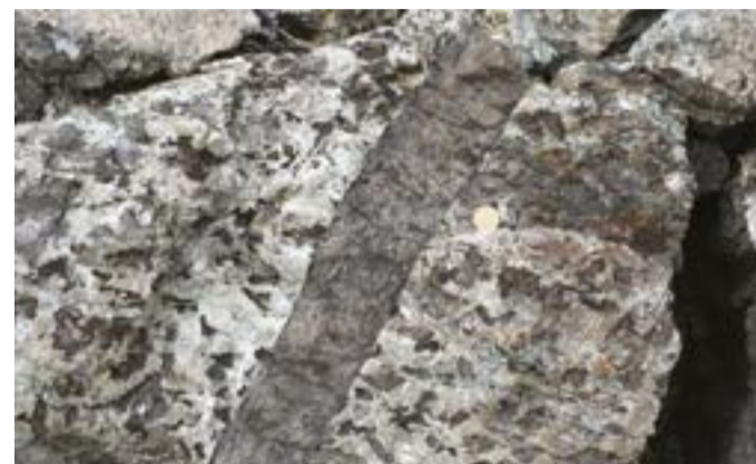
Coarse-grained gabbro, an intrusive igneous rock, cut by a basaltic dike, an effusive igneous rock. Both rock types have typically low U, Th and \text{K}_2\text{O} contents. Source: Roberto Braga.
