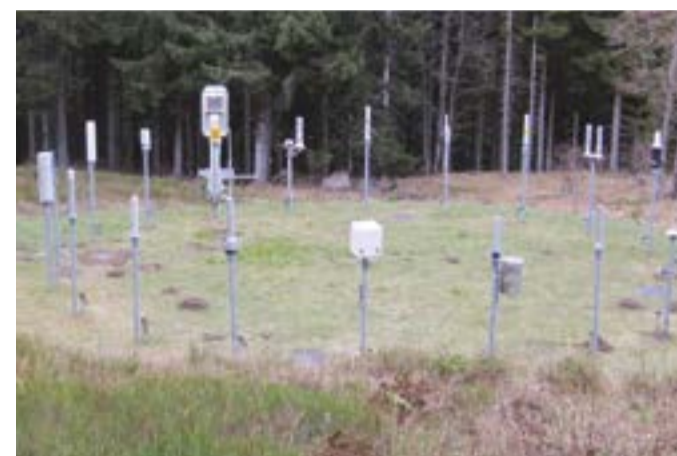
... Dose rate monitors used in European early-warning networks, installed for long-term intercomparisons at the intercalibration site in Schauinsland, Germany. Source: Picture taken from EURAMET (2017).
