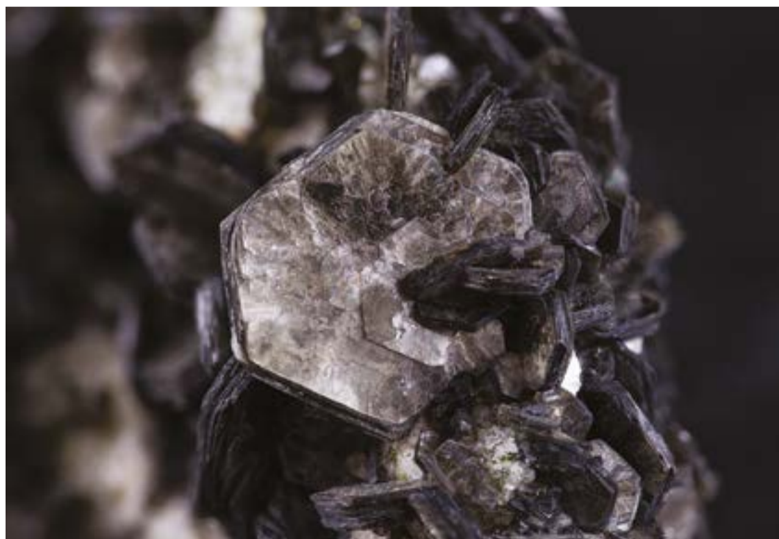
The hexagonal basal section of this white mica from Premia (Antigorio Valley, North Piedmont, Italy) is about 8 mm across. White mica is one of the main rock-forming minerals with a high K content. Source: Sample courtesy of Pietro Grandi (Bologna); photograph by Orlando S. Olivieri.
