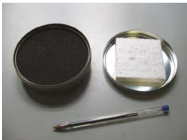
Charcoal canister used to measure indoor radon concentration. Source: Peter Bossew.
