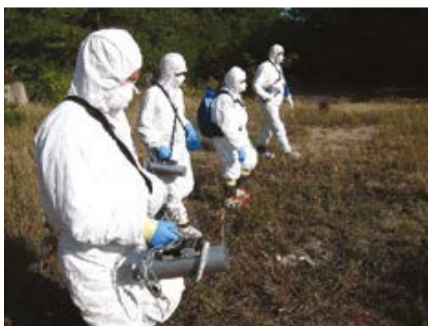
Mobile monitoring. Left: The experimental drone of the German Office for Radiation Protection (BFS), equipped with a CdZnTe detector. Right: 'Walking-borne' and 'Backpack-borne' ground monitoring. Data are automatically geo-referenced and transferred to the base station. Source: Both pictures from an exercise in the Chernobyl exclusion zone, 2016.
