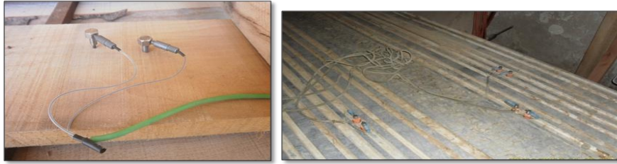
Figure 2. Probe placement for moisture content measurement (convective drying and vacuum drying)
