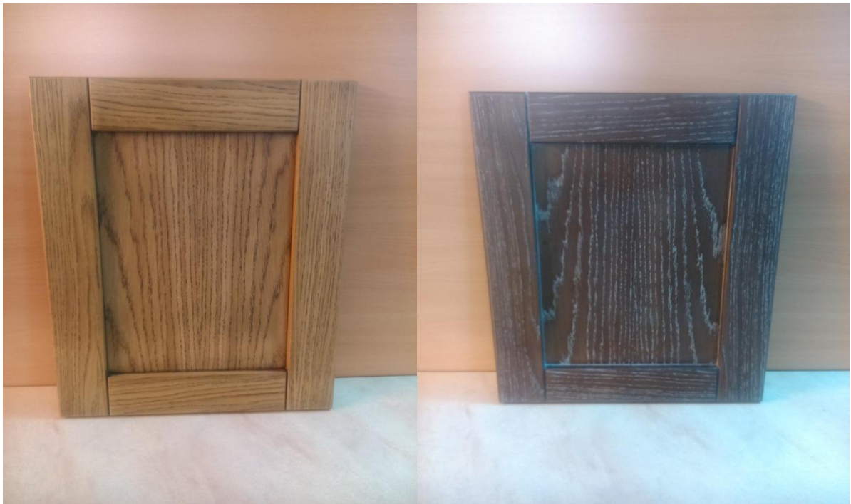
Figure 3. “Black pore “effect (BP) aggregate in left; “White pore” effect (WP) aggregate in right
