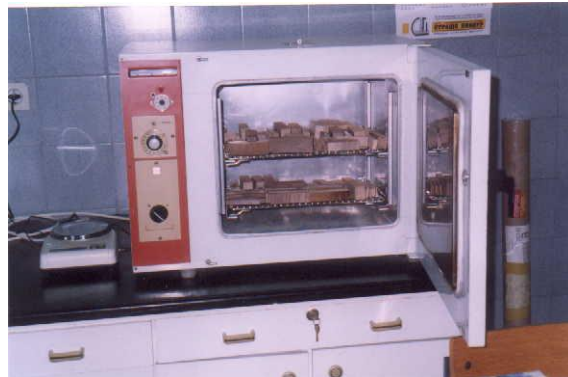
Figure 2. Oven dry method - determination of moisture content distribution
