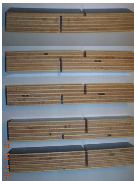
Figure 2. The look of the probes for testing according EN 314
