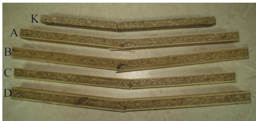
Figure 2. Failure mode of the test specimens of the experimental panels
