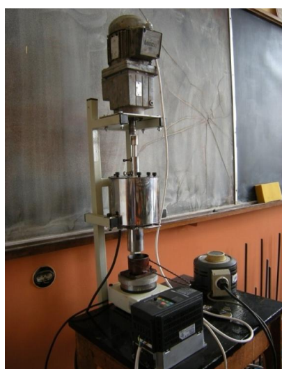
Figure 1. Laboratory apparatus used for wood/carbon dust composite materials production
