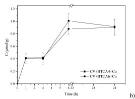
Figure 6: Cu<sup>2+</sup>-ion release from CO and CV fabrics impregnated with CuO/Cu<sub>2</sub>O NPs into physiological saline solution
