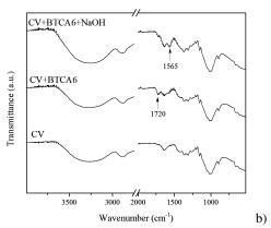
Figure 1: FTIR spectra of (a) control CO sample, CO+BTCA6+Cu sample and Co+BTCA6+Cu sample immersed into 0.1 N NaOH solution; and (b) control CV sample, CV+BTCA6+Cu sample and CV+BTCA6+Cu sample immersed into 0.1 N NaOH solution
